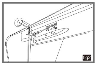
2. Unpack the assessory bag of elevator, which includes servo arms, screws, linkage rods (including clevis and sleeve). Install the servo arms as shown in Figure 3.
