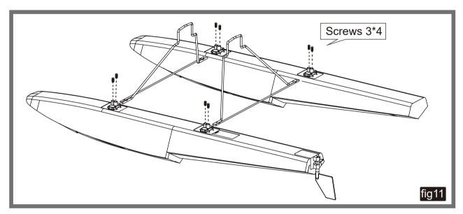
8. Fix the floats set with struts on the bottom of fuselage with screws as shown in Figure 12.
