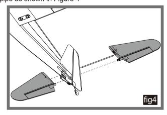
3. Secure the elevator with screws as shown in Figure 5.
