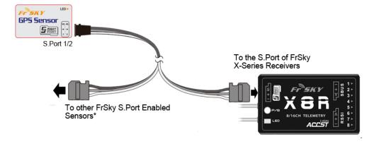
① The GPS should be mounted with Velcro in your model so that the "**UP**' side is facing toward the sky.
