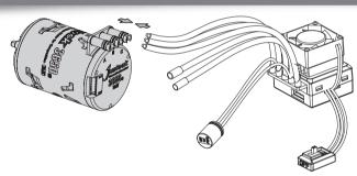
1) Screws used for installation are 3mm in diameter & 5mm in length. Before mounting the motor onto the vehicle, please ensure that all the screws are applicable to avoid damaging the motor. In general it's ok to adopt screws which are 3 mm in diameter and less than 8mm in length; the specific length is up to the chassis size.
