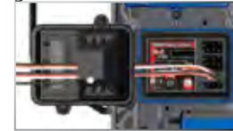
**Note: For best performance, it is recommended that the receiver be installed in the original orientation as shown.**
