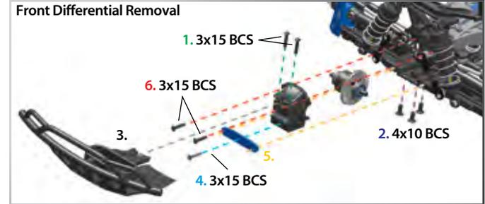
6. Remove two 3x15mm button-head screws from the differential cover. Do not remove the two screws that secure the shock tower.
