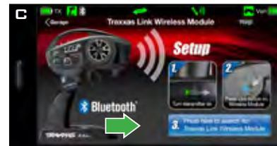
4. Within 10 seconds, touch the "Search for Traxxas Link Wireless Module" button on your mobile device (C).
