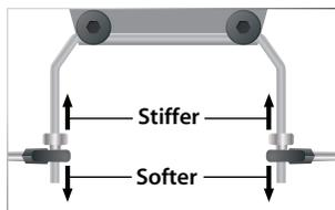
Closer to the pivot point results in a stiffer setup, farther from the pivot point will result in softer sway bar response.
