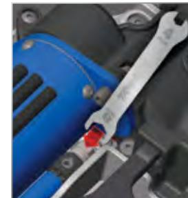
Place the model on a high-traction surface, such as carpet. Adjust the slipper so that you can hear it slip for approximately two feet from a standing, full throttle start. (Learn more about adjusting the slipper clutch in the sidebar.)
