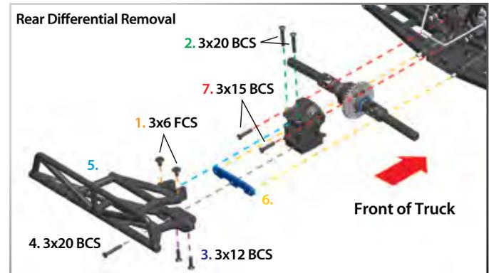
5. Slide the bumper assembly off of the chassis.
