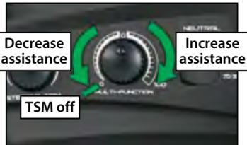
**Note:** TSM is deactivated automatically when driving or braking in reverse.
