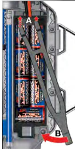
Install the battery pack with the battery wires facing the rear of the model. Insert the tabs of the battery hold-down into the slots in the rear hold-down retainer (A). Swing the battery hold down towards the chassis and snap (lock) the end into the front hold-down retainer (B).
