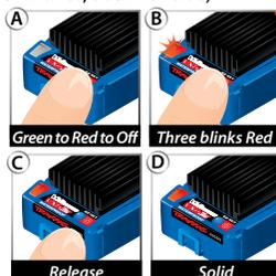
**Note:** If you missed the mode you wanted, keep the EZ-Set button pressed down and the blink cycle will repeat until the button is released and a Mode is selected.
