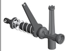
**A. Tighten/Loosen Upper Cap**
