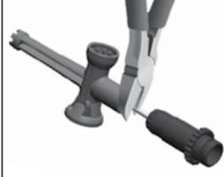
**C. Remove/Install Rod End**
