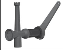
**B. Tighten/Loosen Lower Cap**
