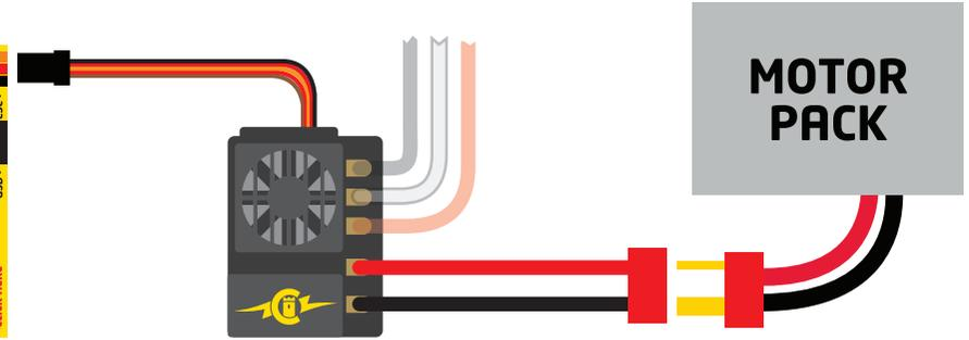
Field Link and ESC are both powered by the motor pack
