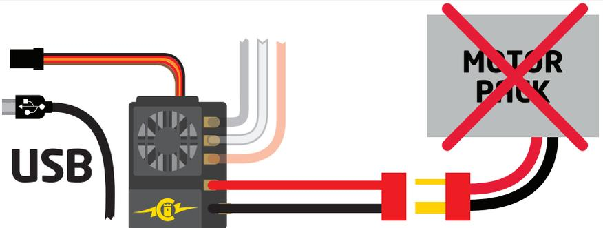
Field Link and ESC are both powered by the USB connection
