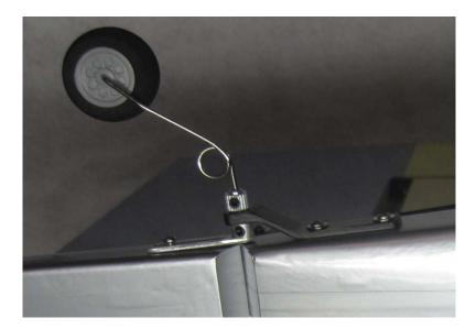
21. Place the tailwheel wire in the proper position, aligned with the rudder and lock into place with the 2 set screws.
