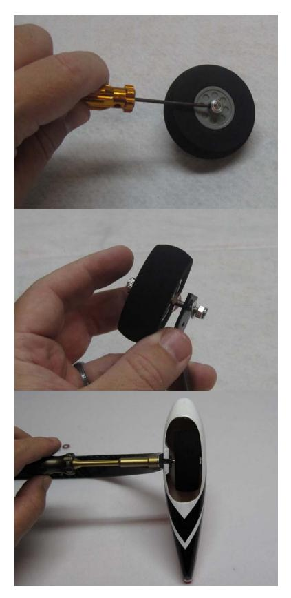
12. Secure the landing gear to the fuselage by inserting a 3mm bolt into a washer, through the carbon fiber gear and into the pre-installed blind nuts in the fuselage. Make sure to use a drop of blue Loctite on each bolt to prevent them from backing out.
