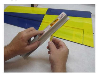
3. Use a sharp hobby blade to remove the covering 1/16 of an inch inside the line you traced around the control horn base.
