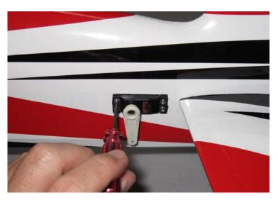
23. The rudder and elevator servo linkages assemble and are installed just like the aileron linkages. For maximum control surface travel we highly recommend using the Long Dubro Super Strength servo arms. (Dubro part #670 for Futaba, #671 for JR and #672 for Hitec)
