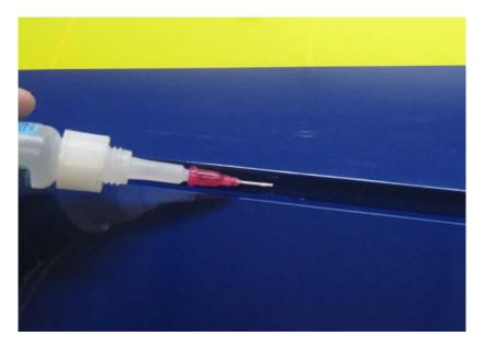
17. Insert the stabilizer into its slot and the carbon fiber wing tube into the fiberglass sleeve. Use a ruler to insure that the stabilizer is centered in its slot and compare the stabilizer to the wing tube to make sure it is properly aligned. Sand or shim the slot if necessary to ensure proper alignment. Secure the stabilizer with CA.
