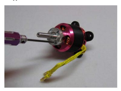
27. Mount the Torque motor using the supplied 3mm black socket head cap bolts and washers. The bolts are to be inserted into the blind nuts which are pre-installed in the motor mount plate. Be sure to put a drop of blue Loctite onto each bolt to prevent them from backing out. <u>Be sure to add some CA to all motor box joints!</u>
