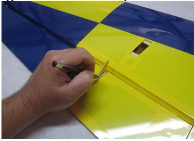
2. Remove the control horn and scuff the portion that will be glued into the aileron with sandpaper.
