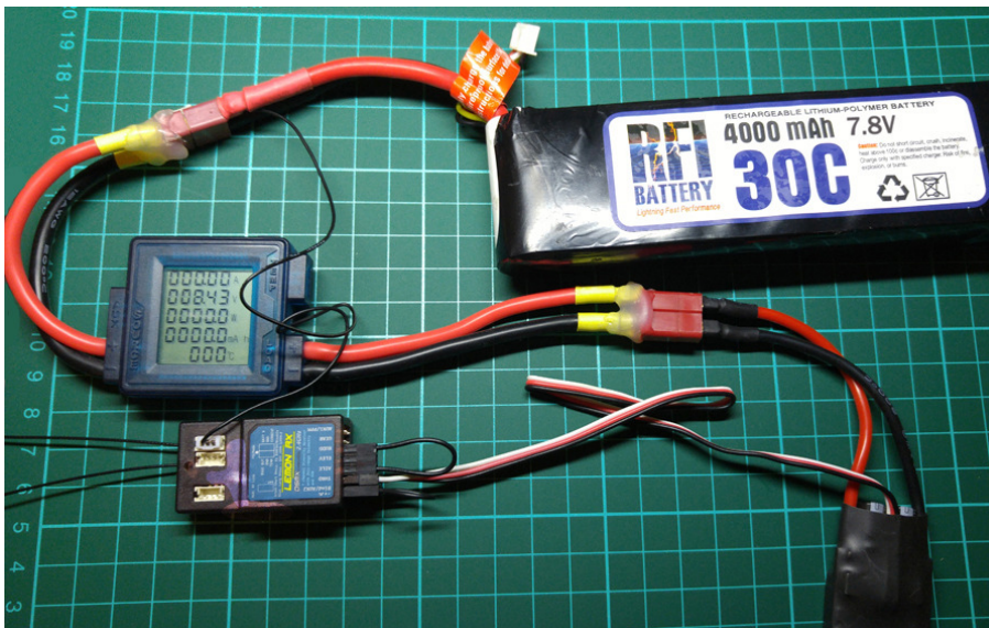
Figure 5.2 – Voltage sensor calibrated at 8.4V. The green device is a voltage and current measurement device (Wattmeter) to confirm the actual battery voltage.
