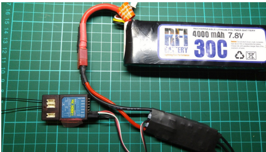
Figure 2.2 – Solid red light indicates successful binding
