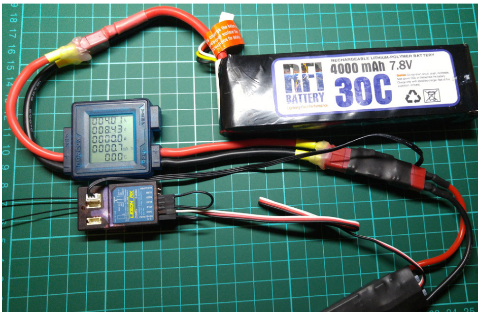
Figure 6.2 – V/I sensor calibrated at 8.4V and 4A. The green device is a wattmeter to confirm the actual battery voltage and current.
