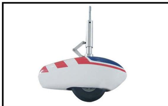
2) Install landing gear at the top Fuselage.
