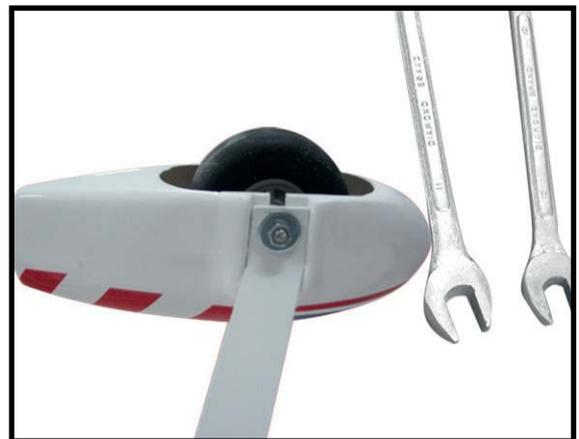
3) A drop of C/A glue on the wheel collar screws will help keep them from coming loose during operation.
