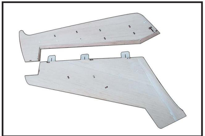
Sanding rounded leading edge area of fin until the shape seamless as (photo 19).
