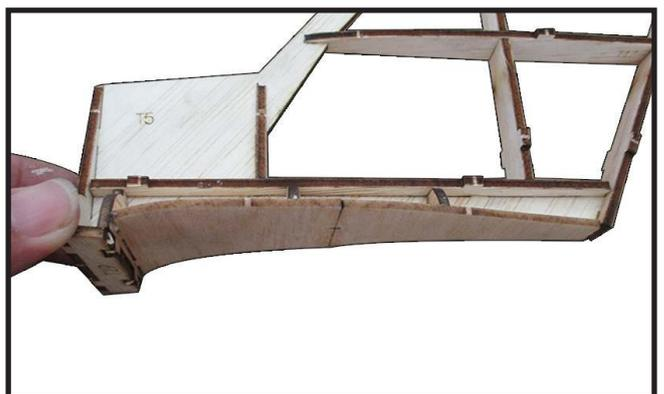
Locate and apply sheet T23 (2pcs) at two sides as (photo 8).
