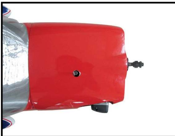
2) While keeping the back edge of the cowl flush with the marks, align the front of the cowl with the crankshaft of the engine. The front of the cowl should be positioned so the crankshaft is in **nearly** the middle of the cowl opening. Use the spinner backplate as a guide. Hold the cowl firmly in place using pieces of masking tape.
