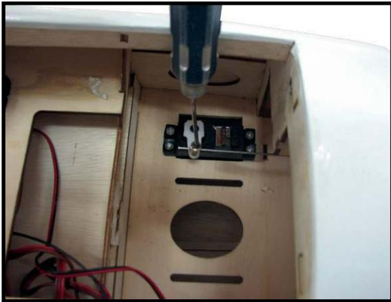
8) Move the throttle stick to the closed position and move the carburetor to closed. Use a 2.5mm hex wrench to tighten the screw that secures the throttle pushrod wire. Make sure to use threadlock on the screw so it does not vibrate loose.
