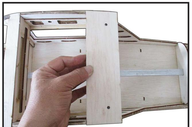
Locate and cover balsa sheet H6 on top hatch as (Photo 88).
