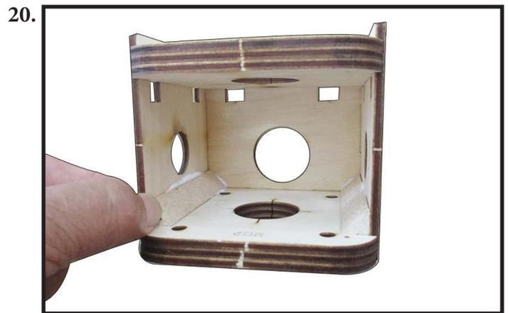
Locate and assemble 5 pieces to become the motor mount box (Photo 19).
