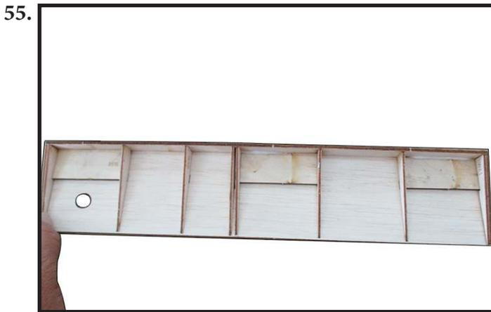
Locate and apply W1 to W2. And then set up wing to fuselage by sanding until fitting (no gap between wing and fuselage). (Photo 58).
