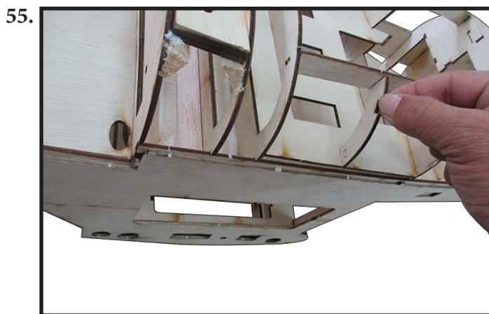
Locate and assemble F34 (the mount of strut) at left side and right side as (Photo 56).
