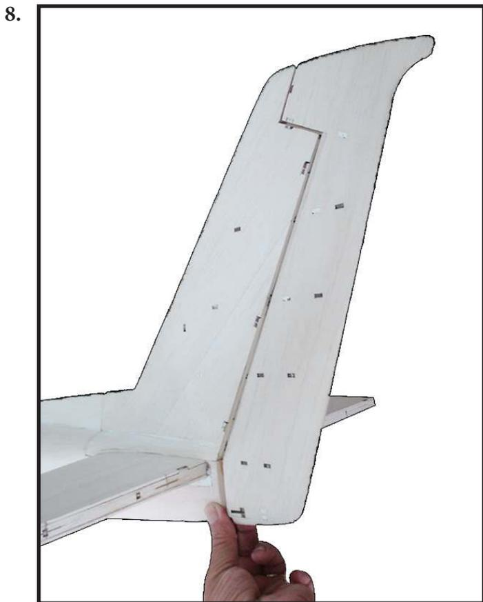
Sanding rounded bottom of rudder so that it look like seamless with fuselage.
