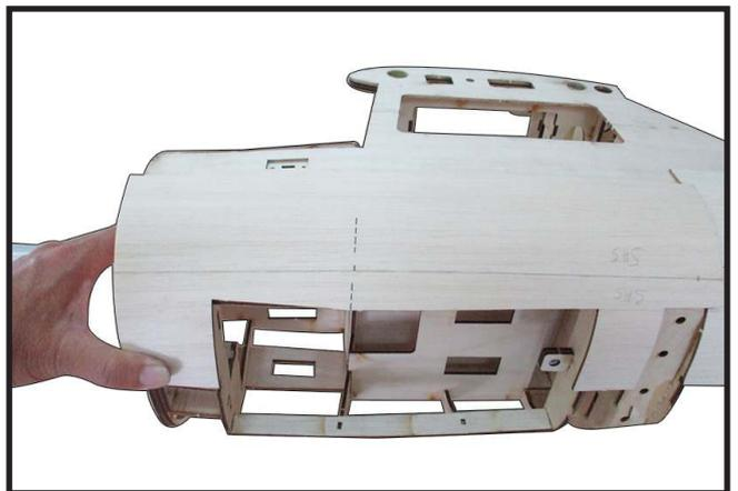
Weld together two difference pieces SH1 become a sheet (left and right) by CA glue as photo shown. (photo 81,82).
