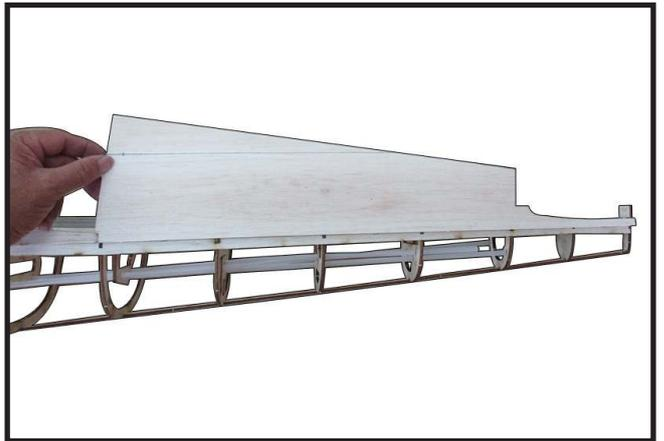
Weld together two difference pieces SH3 become a sheet (left and right) by CA glue as photo shown. (photo 74,75).
