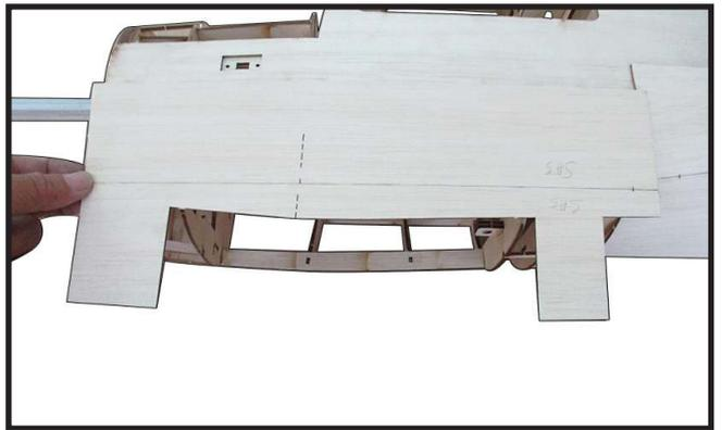
Bend the balsa sheet SH5 go to bottom area and toward area. Then, add CA glue and use the finger at this place until the glue dries as photo shown.
