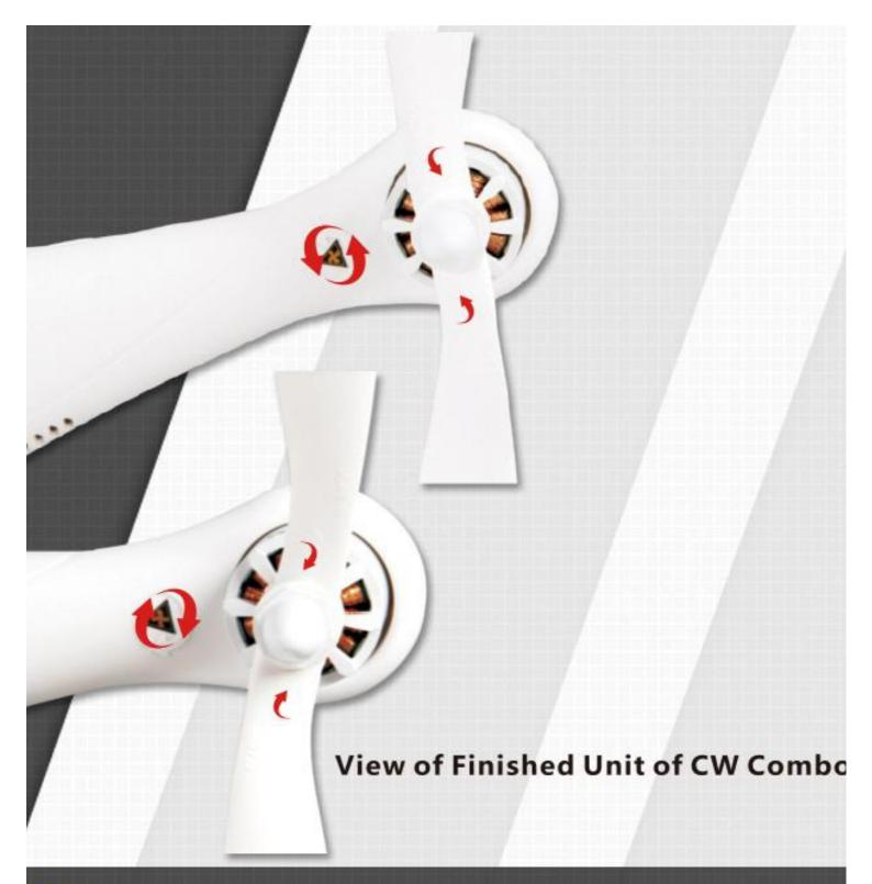
NOTE: A trial test is required before flying. Follow the illustrations above for testing directions of rotation... If the rotors rotate in reverse, it will be necessary for you to reverse motor's connecting wires. When a separated ESC is applied to installation you are also required to reverse the motor's connecting wires.
