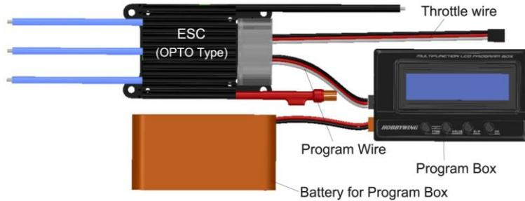
1.2 Step B: Connect ESC to battery and switch it on.
