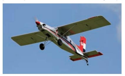
The struttery is what lets this model down. The tubes have flattened ends which are positive weak points.
