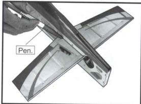
☐ 3) Remove the horizontal. Using the lines you just drew as a guide, carefully remove the covering from between them using a modeling knife.
