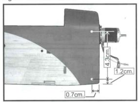
□ 2) Slide the fiberglass cowl over the engine and line up the back edge of the cowl with the marks you made on the fuselage then trim and cut.
