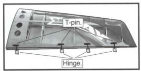
□ 3) Slide the wing panel on the aileron until there is only a slight gap. The hinge is now centered on the wing panel and aileron. Remove the T-pins and snug the aileron against the wing panel. A gap of 1/64" or less should be maintained between the wing panel and aileron.
