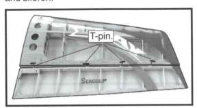
□ 4)Deflect the aileron and completely saturate each hinge with thin C/A glue. The ailerons front surface should lightly contact the wing during this procedure. Ideally, when the hinges are glued in place, a 1/64" gap or less will be maintained throughout the lengh of the aileron to the wing panel hinge line.
