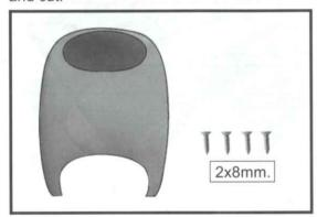
□ 3) While keeping the back edge of the cowl flush with the marks, align the front of the cowl with the crankshaft of the motor. The front of the cowl should be positioned so the crankshaft is in **nearly** the middle of the cowl opening. Use the spinner backplate as a guide. Hold the cowl firmly in place using pieces of masking tape.
