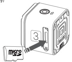
**NOTICE:** Use care when handling memory cards. Avoid liquids, dust, and debris. As a precaution, power off the camera before inserting or removing the card. Check manufacturer guidelines regarding use in acceptable temperature ranges.
