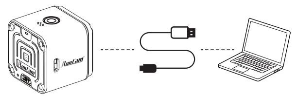
After being connected to the computer by a USB cable, the camera is in MSDC mode. Press the Power/Shutter button to switch to WebCam mode.
