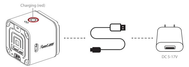
The RunCam 3 uses internal battery. After powering on, if the battery is more than 50% charged, the camera status lights (green) will blink 5 times. If the battery is less than 50% charged, the camera status lights (green) will blink 10 times. If the battery drops below 15%, the camera status lights (green) will blink continuously.
