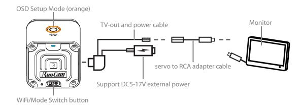
After powering on, long press the WiFi/Mode Switch button until the camera status lights become orange. The camera is now in the OSD setup mode. In the OSD setup mode, use the provided "USB Video Power Cable" to connect the camera to a monitor and make settings on the screen.
